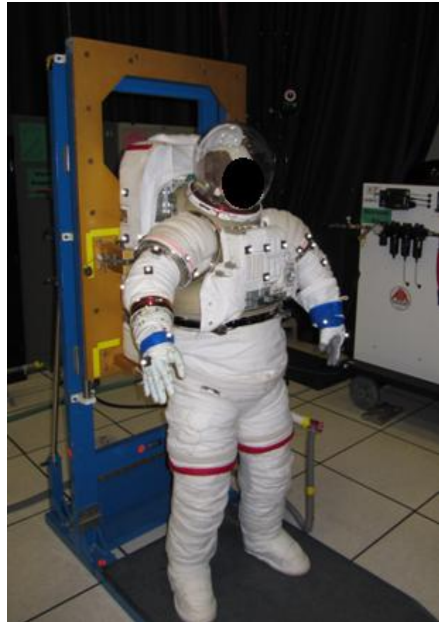
EMU attached to Suit-Donning Stand with Thermal Micrometeorite Garment removed from HUT
